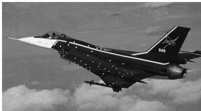
Fig. 2 F-16XL-1 aircraft with missiles, tufts, modified flow-visualization paint scheme, and video targets (NASA photo EC96-43508-2).
